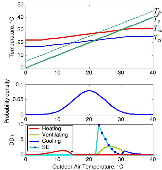
Fig. 3 Climate suitability: a) comfort zone and free running temperature; b) probability density distribution of outdoor air temperature; c) probability distribution of degree-time.
