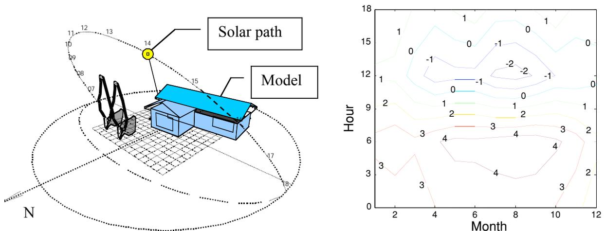
Fig. 2 a) Model of building obtained by using ECOTECT software. b) Temperature difference between inside and outside temperature obtained for the model using weather data for Athens.
