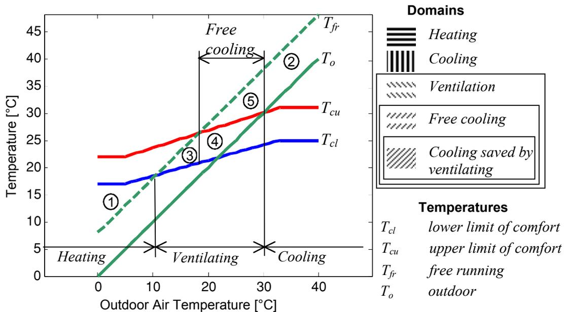
Fig. 1 Heating, ventilating and cooling domains.
